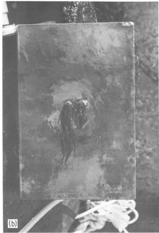
Figure 13 Surface condition of (a) P.V.C. control sample, (b) freely corroding copper plate and (c) spiked copper plate after 110 days exposure at the Fawley site.
